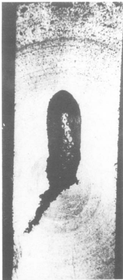
Figure 7 Macrophotograph of longitudinal section of aluminium alloy-mica particle composite casting poured in a sand mould with heavy copper chill at the top ( \times 0.85 ).
